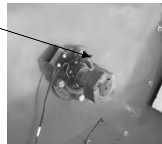
Transition auger drive jack shaft one on each side.
