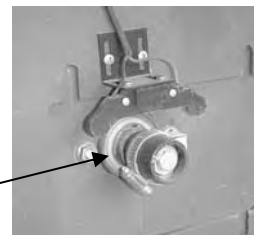
Auger Shaft sensor
