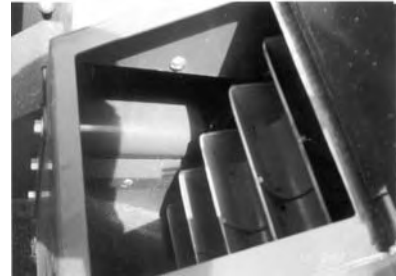
Conveyor Belt-Bucket elevator Chamber
