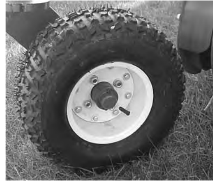
Pickup head tire Tire size-18 x 9.0-8 Maintain 10 lbs. pressure
