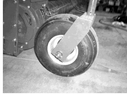
Pickup head tire Tire size-18 x 9.5-8 Maintain 24 lbs. pressure
