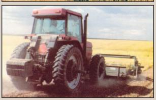
The front tractor weights can be transferred to the rear 3 points to distribute weight evenly throughout the entire tractor.
