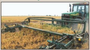
Mounted on each side of the machine are heavy duty scissor type gauge wheels with dividers. They provide precise rod depth control & smooth vine separation.
