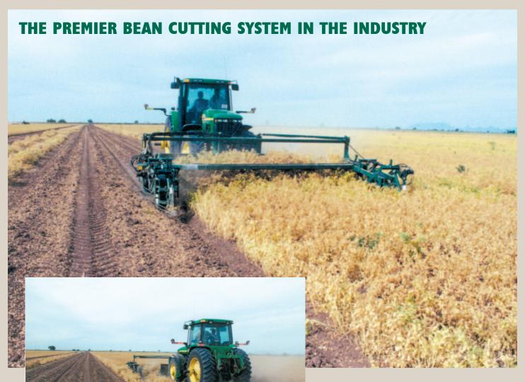
The design of the One Step<sup>TM</sup> Ahead will allow pulling and windrowing of row crops or solid seeded crops in one operation with virtually no loss.
